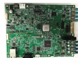
R-Car V3H reference design including Renesas PMICs and 5P35023 Timing IC
